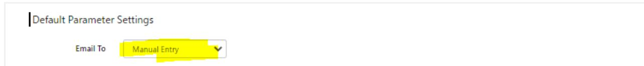
With this option selected, in workflow application Email address can be entered manually using softkey board on MFP Operation Panel.
